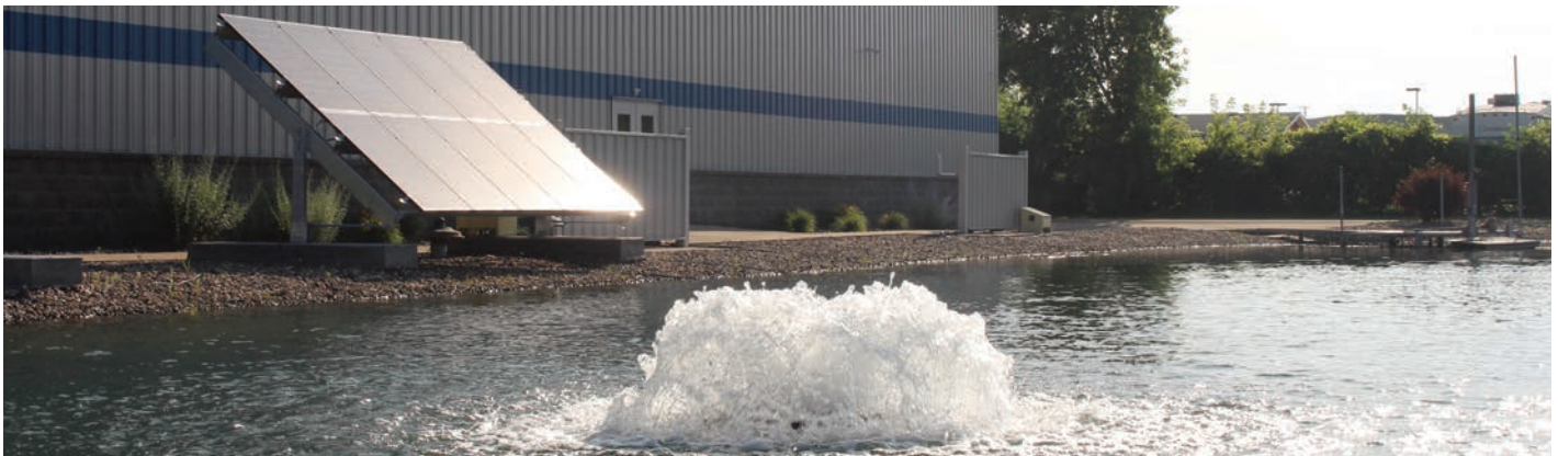
2HP Surface Aerator running on all 10 solar panels in Wisconsin
